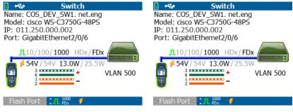
1 Gigabit link on copper with PoE on port 6 1 Gigabit link on fiber on port 38
